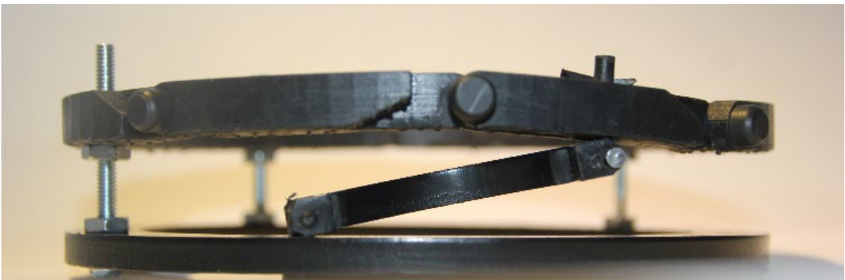
Figure 3.11: The hinge joints used in the mechanism.
