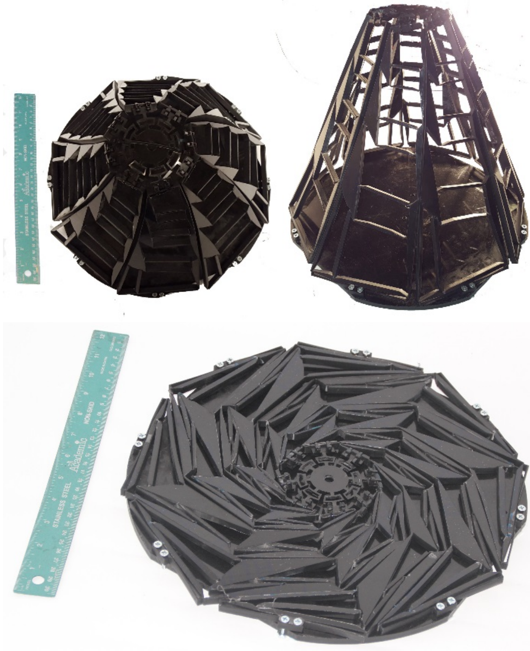
Figure 5.18: Lamina Emergent Frustum in both stable positions. The planar position and frustum position (top and side views).
